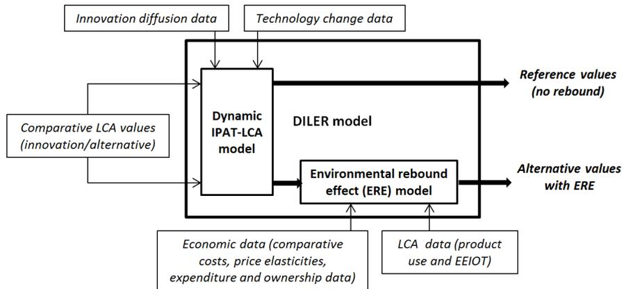
**Figure 1.** Graphic overview of the DILER model. Bolded boxes represent models, whereas non-bolded boxes represent data inputs. Bolded arrows represent endogenous modelled data flows, whereas non-bolded arrows represent literature data flows. LCA: life cycle assessment, EEIOT: environmentally extended input-output table.
