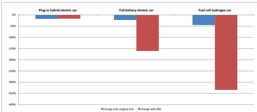
**Figure 5.** Comparative results between original LCA scores and LCA scores considering the environmental rebound effect (ERE) (in CO<sub>2</sub> eq.) for various electric propulsion technologies for passenger cars.
